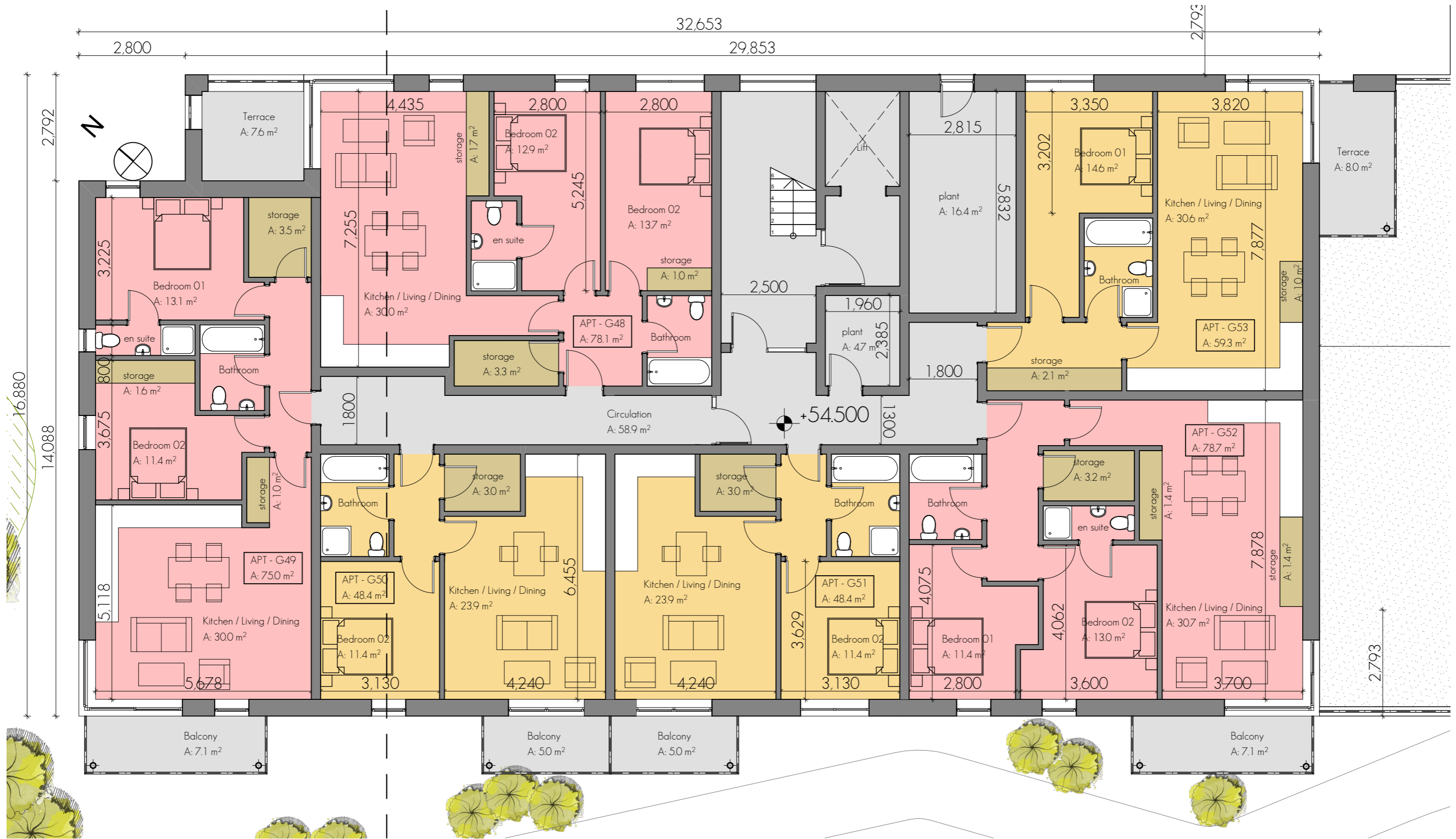
LOWER GROUND FLOOR PLAN - BLOCK B - LEVEL_54.500 1:100
