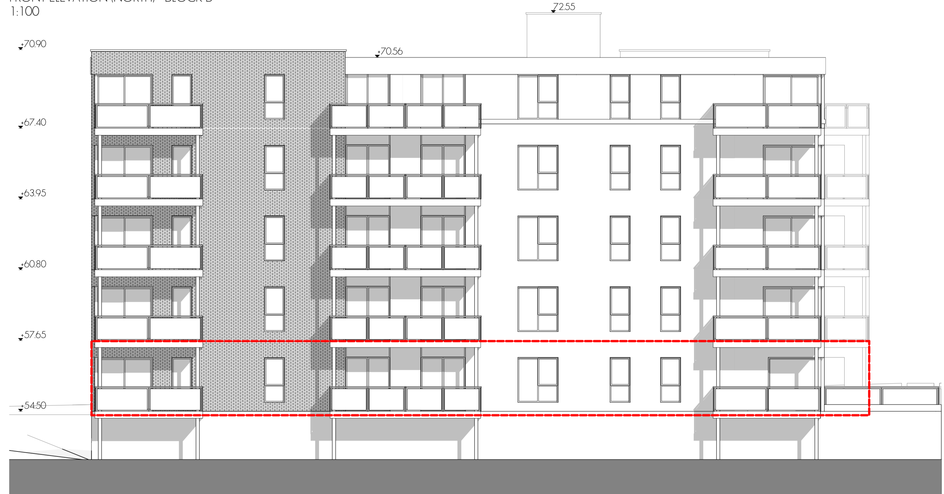
REAR ELEVATION (SOUTH) - BLOCK B 1:100
